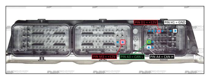
WARNING: due to the relevant power absorbed by the ECU at the beginning of the communication we suggest to feed the ECU with an external power supply or a car battery. Connect the power cable F32GN003 to the Trasdata and then to the power source.
