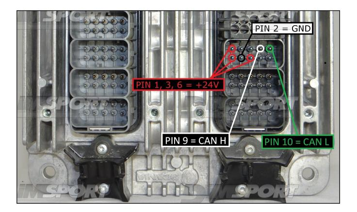
To the power feeding pins 1,3,6 (+24V) you can connect both wires red (VECU) and orange (VKEY) of the F32GN037C/D cable.
