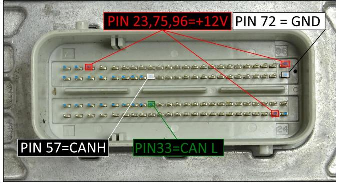
To the power feeding pins 23,75,96 (+12V) you can connect both wires red (VECU) and orange (VKEY) of the F32GN037C/D cable, they both have 12V signal.
