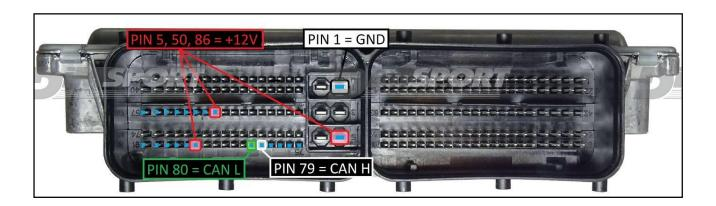
To the power feeding pins 5,50,86 (+12V) you must connect only the red wires (VECU) of the F32GN037C cable.
