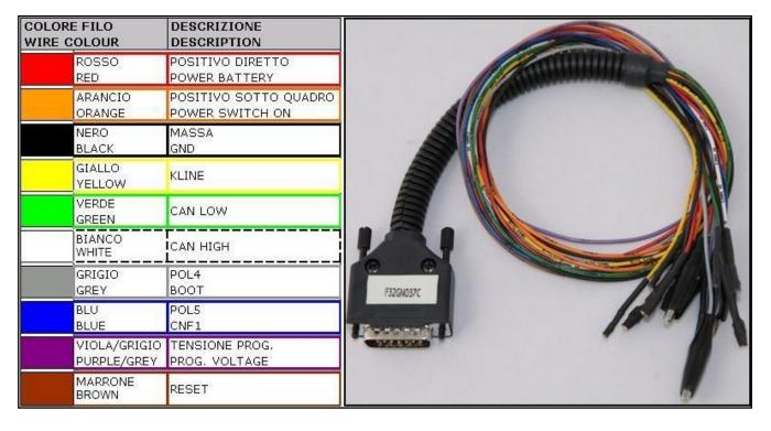
Due to the relevant power absorbed by the ECU at the beginning of the communication procedures it is necessary to feed the ECU with a booster or an additional battery. The ECU must be fed through the Trasdata, connect the F32GN003 power cable to the Trasdata.
