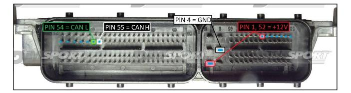
WARNING: due to the relevant power absorbed by the ECU at the beginning of the communication we suggest to feed the ECU with an external power supply or a car battery. Connect the power cable F32GN003 to the Trasdata and then to the power source. The ECU must be powered through the Trasdata using the F32GN0037C cable
