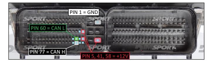
To the power feeding pins 5,41,58 (+12V) you can connect both wires red (VECU) and orange (VKEY) of the F32GN037C/D cable, they both have 12V signal.
