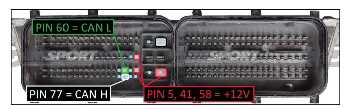
To the power feeding pins 5,41,58 (+12V) you can connect both wires red (VECU) and orange (VKEY) of the F32GN037C cable, they both have 12V signal.
