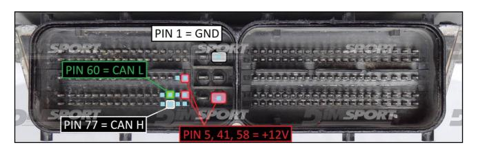
To the power feeding pins 5,41,58 (+12V) you can connect both wires red (VECU) and orange (VKEY) of the F32GN037C/D cable, they both have 12V signal.
