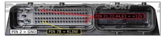
To pin 21,22,44,63 it is possible to connect RED and ORANGE wires, they both are 12V
