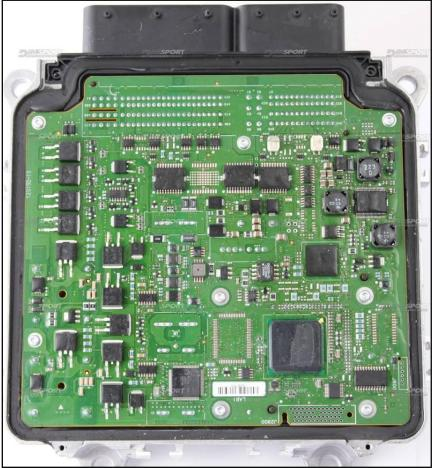
The lay-by pins are placed in the lower part of the ECU **WARNING**: solder the wires without creating any short circuits among the pads.
