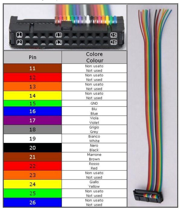
Please avoid short circuits while soldering the wires on the pads
