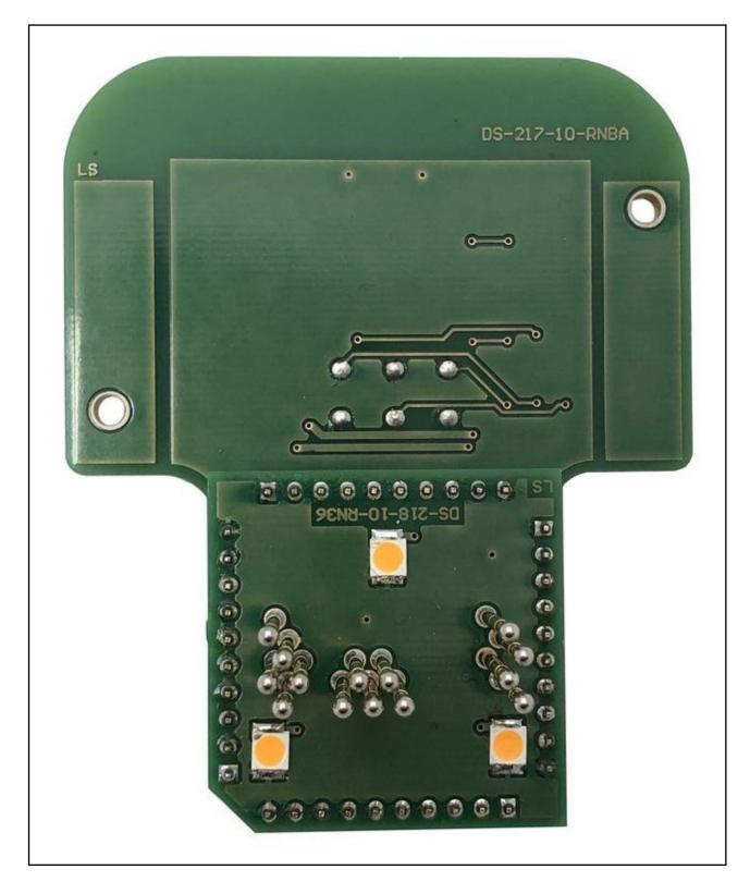
Verify the PIN 1 location and connect the pin 18/BOT to the corresponding clamp on the base adapter F34DM036 as in displayed in the following picture. Place F34DM036+F34DM037 adapters as displayed in the following picture.
