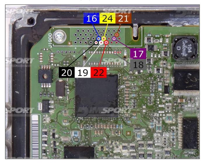
Connect the wires on the pads avoiding any short circuits.
