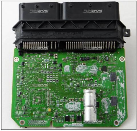
In order to connect to the ECU use the CABLE F32GN037C/D. Make sure that the POWER led (red) on Trasdata is ON.
