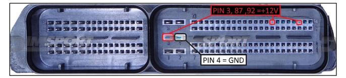
To the power feeding pins 3,87,92 (+12V) you can connect both wires red (VECU) and orange VKEY) of the F32GN037C cable, they both have 12V signal.
