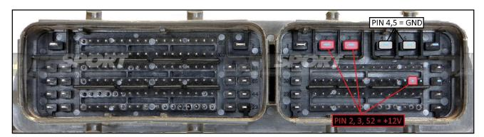
To the power feeding pins 2,3,52 (+12V) you can connect both wires red (VECU) and orange VKEY) of the F32GN037C cable, they both have 12V signal.
