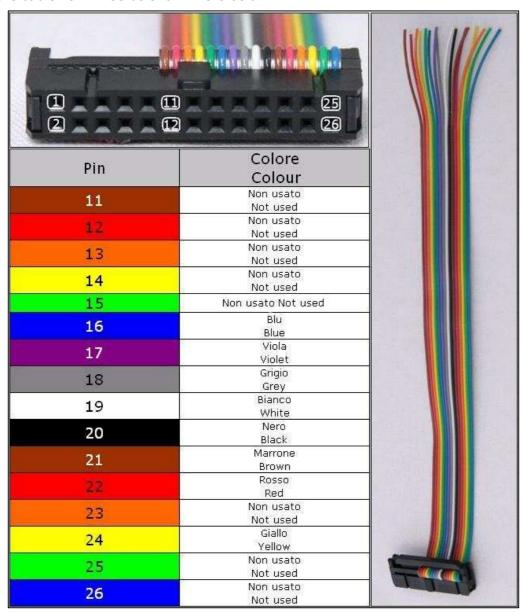
**WARNING:** connect the wires avoiding any short circuits among the pads.
