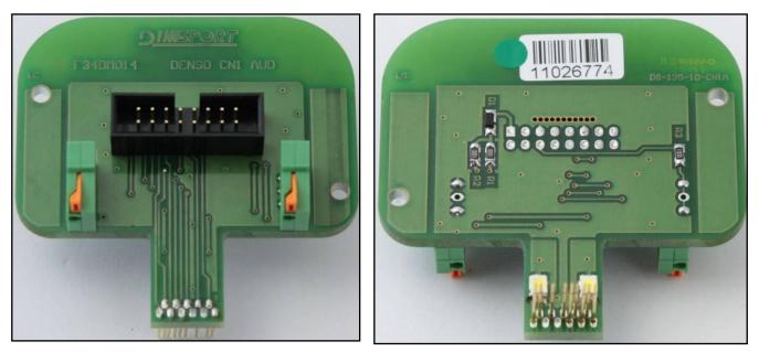
**WARNING**: while connecting the adapter F34DM014 take care of the PIN1 assignment.
