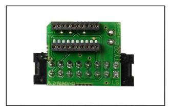
By using the grey wire supplied with the adapter connect the pad 18 (see pg.7) to the specific connector on the adapter itself.
