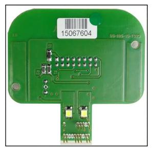
By using a wire connect the pad 18 (see pg.7) to the specific orange clamp ENA present on the  $F34DM023\ DIMA\ adapter$ .
