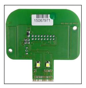
By using a wire connect the pad 18 (see pg.5) to the specific orange clamp ENA present on the  $F34DM024\ DIMA\ adapter$ .
