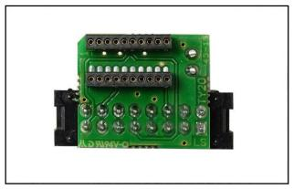
By using the grey wire supplied with the adapter connect the pad 18 (see pg.6) to the specific connector on the adapter itself.
