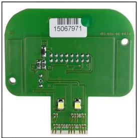
By using a wire connect the pad 18 (see pg.5) to the specific orange clamp ENA present on the F34DM024 adapter.
