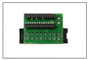
By using the grey wire supplied with the adapter connect the pad 18 (see pg.5) to the specific connector on the adapter itself.
