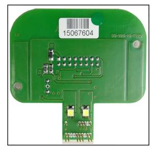
By using a wire connect the pad 18 (see pg.8-9) to the specific orange clamp ENA present on the F34DM023 DIMA adapter.
