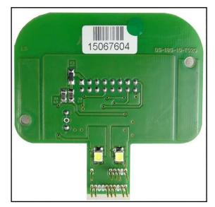
By using a wire connect the pad 18 (see pg.8) to the specific orange clamp ENA present on the F34DM023 DIMA adapter.
