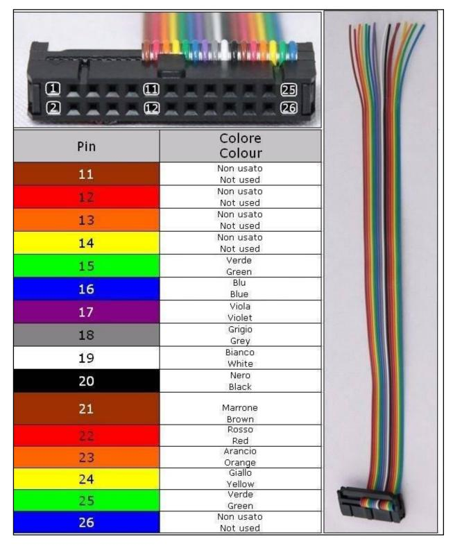
**WARNING:** the grey wire can be connected in two different ways to the pin 18: 1) directly soldered on the pad present on the upper side of the board
