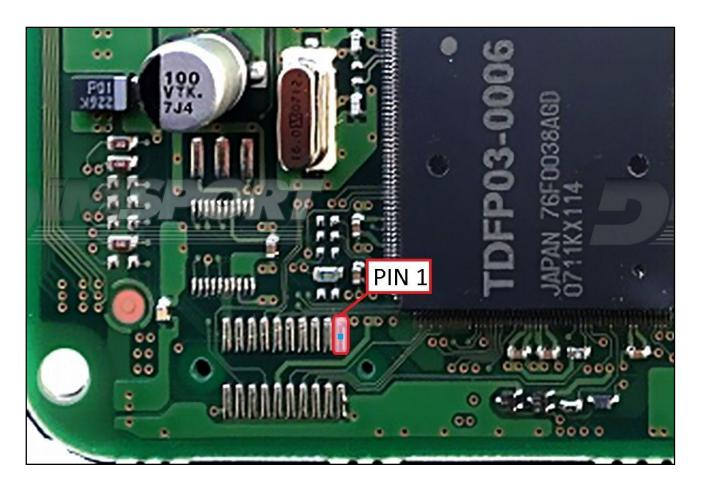
Identify the pin n.18 for the grey wire connection in order to enable the communication with the microprocessor, as explained in the following pages.
