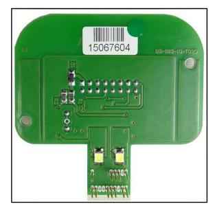
By using a wire connect the pad 18 (see pg.5) to the specific orange clamp ENA present on the F34DM023 DIMA adapter.
