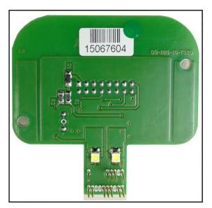
By using a wire connect the pad 18 (see pg.6) to the specific orange clamp ENA present on the F34DM023 DIMA adapter.
