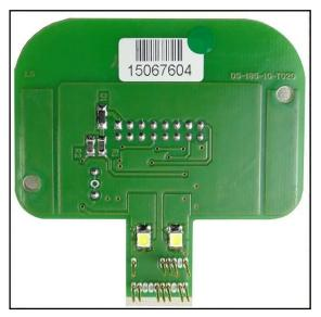
By using a wire connect the pad 18 (see pg.5) to the specific orange clamp ENA present on the F34DM023 DIMA adapter.
