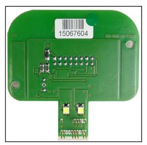
By using a wire connect the pad 18 (see pg.5) to the specific orange clamp ENA present on the F34DM023 adapter.
