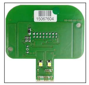
By using a wire connect the pad 18 (see pg.6) to the specific orange clamp ENA present on the F34DM023 adapter.
