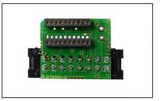
By using the grey wire supplied with the adapter connect the pad 18 (see pg.8-9) to the specific connector on the adapter itself.
