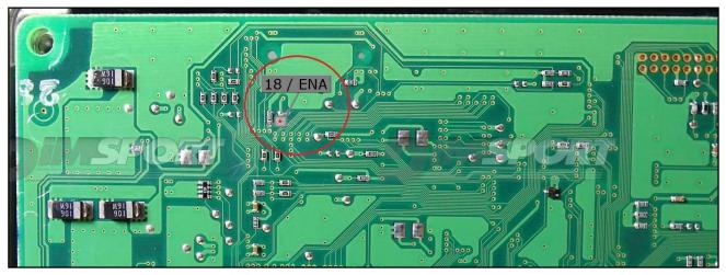
1) microclamp connected on the microprocessor then connect the grey wire 18 to the microclamp. (check the example picture here below)
