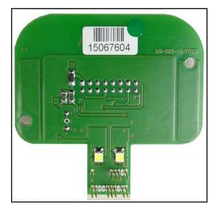
By using a wire connect the pad 18 (see pg.6) to the specific orange clamp ENA present on the F34DM023 DIMA adapter.
