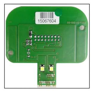
By using a wire connect the pad 18 (see pg.6) to the specific orange clamp ENA present on the F34DM023 adapter.
