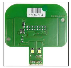
By using a wire connect the pad 18 (see pg.5) to the specific orange clamp ENA present on the F34DM023 adapter.
