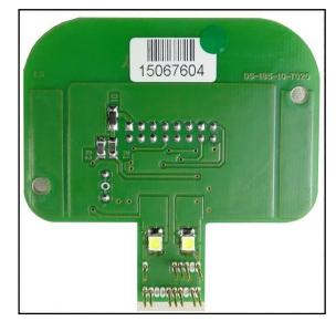
By using a wire connect the pad 18 (see pg.8-9) to the specific orange clamp ENA present on the F34DM023 adapter.
