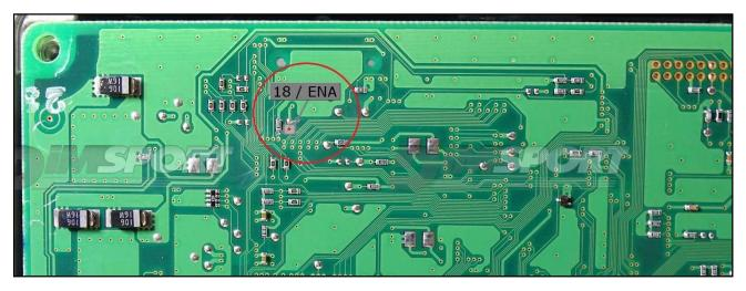
2) microclamp connected on the microprocessor then connect the grey wire 18 to the microclamp. (check the example picture here below)
