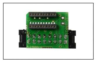
By using the grey wire supplied with the adapter connect the pad 18 (see pg.5) to the specific connector on the adapter itself.
