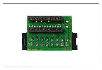
By using the grey wire supplied with the adapter connect the pad 18 (see pg.6) to the specific connector on the adapter itself.
