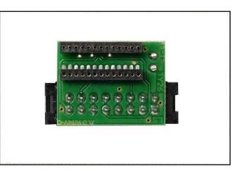
By using the grey wire supplied with the adapter connect the pad 18 (see pg.9) to the specific connector on the adapter itself.
