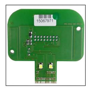
By using a wire connect the pad 18 (see pg.9) to the specific orange clamp ENA present on the F34DM024 DIMA adapter.
