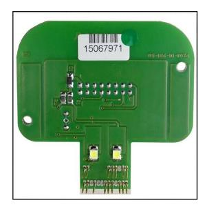
By using a wire connect the pad 18 (see pg.6) to the specific orange clamp ENA present on the F34DM024 DIMA adapter.
