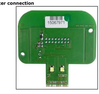
By using a wire connect the pad 18 (see pg.8) to the specific orange clamp ENA present on the F34DM024 adapter.
