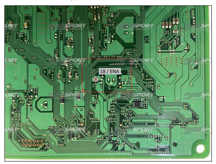
**WARNING :** the grey wire 18 must be connected to the pad placed on the backside of the board, as shown in the following picture.
