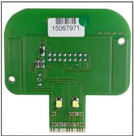
By using a wire connect the pad 18 (see pg.7) to the specific orange clamp ENA present on the F34DM024 adapter.
