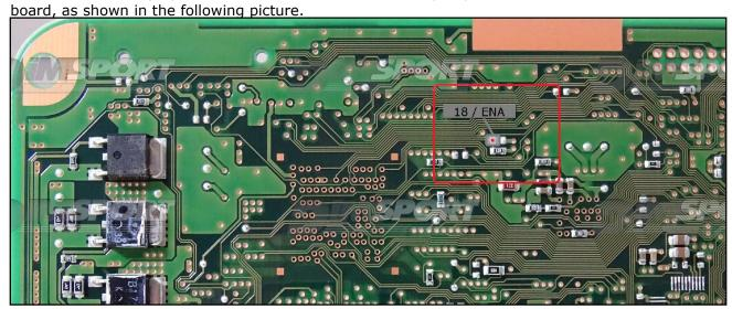
**WARNING:** for a correct reading and writing operation it is necessary to perform a LINK between the pads displayed in the picture here below. Remove the LINK before placing back the ECU into the car.
