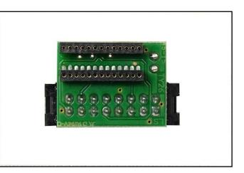
By using the grey wire supplied with the adapter connect the pad 18 (see pg.8) to the specific connector on the adapter itself.
