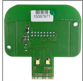
By using a wire connect the pad 18 (see pg.8) to the specific orange clamp ENA present on the F34DM024 DIMA adapter.
