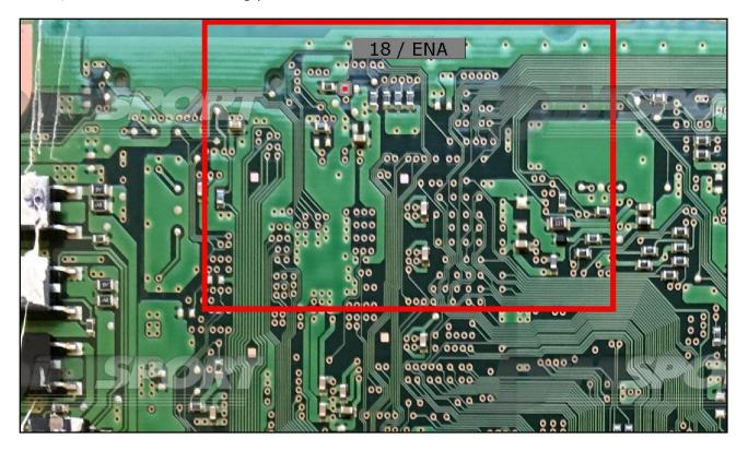
**WARNING**: for a correct reading and writing operation it is necessary to perform a LINK between the pads displayed in the picture here below. Remove the LINK before placing back the ECU into the car.
