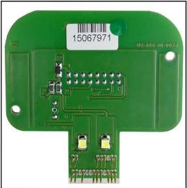
By using a wire connect the pad 18 (see pg.8) to the specific orange clamp ENA present on the F34DM024 adapter.
