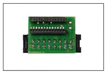
By using the grey wire supplied with the adapter connect the pad 18 (see pg.7) to the specific connector on the adapter itself.
