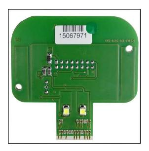
By using a wire connect the pad 18 (see pg.7) to the specific orange clamp ENA present on the  $F34DM024\ DIMA\ adapter$ .
