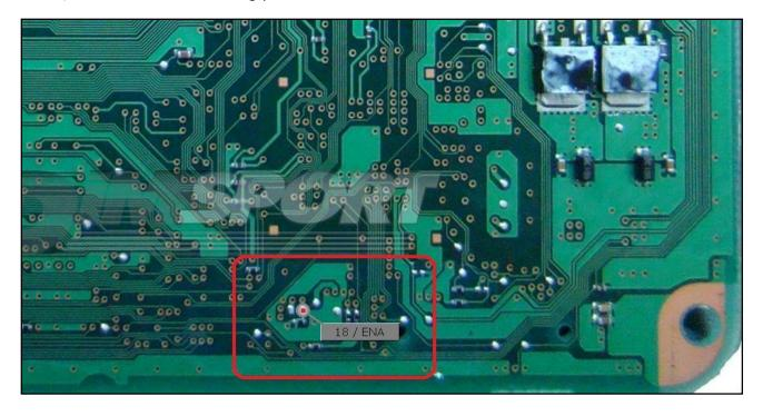
**WARNING**: for a correct reading and writing operation it is necessary to perform a LINK between the pads displayed in the picture here below. Remove the LINK before placing back the ECU into the car.
