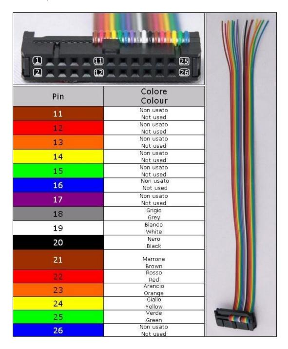
For a correct soldering procedure clean very well the soldering lay-by pins from the plastic film. We suggest you to use fine grit glass-paper smoothing by gentle pressure the connection lay by pins.
