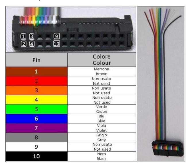
For a correct soldering procedure clean very well the soldering lay-by pins from the plastic film. We suggest you to use fine grit glass-paper smoothing by gentle pressure the connection lay by pins.
