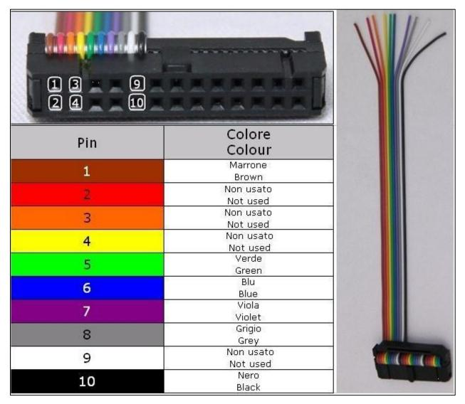
For a correct soldering procedure clean very well the soldering lay-by pins from the plastic film. We suggest you to use a fine grit glass-paper smoothing by gentle pressure the lay by pins connection.
