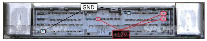
To the power feeding pins +12V you can connect both wires red (VECU) and orange VKEY) of the F32GN037C cable, they both have 12V signal.
