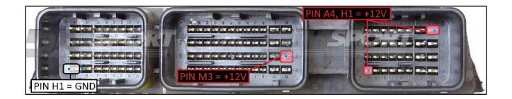
To the power feeding pins M3,A4,H1 ( $\pm$ 12V) you can connect both wires red (VECU) and orange VKEY) of the F32GN037C cable, they both have 12V signal.
