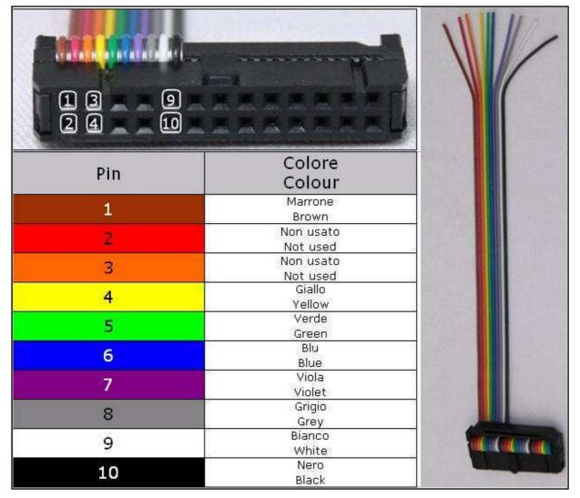
For a correct soldering procedure clean very well the soldering lay by pins from the plastic film. We suggest you to use a fine grit glass paper smoothing by gentle pressure the connection of the lay by pins.
