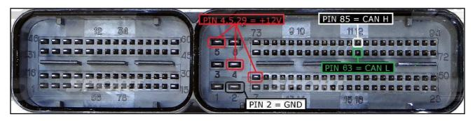
To the pin 4,5,29 connect all +12V RED wires, or it is possible to use one orange wire connected to pin 29.
